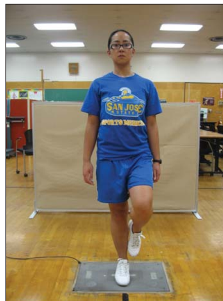
FIGURE 6. Balance was measured on the force plate during single-limb standing. Subjects stood for 20 seconds on the foot with chronic ankle instability, focusing on a 10-cm-diameter circle placed 3 m away at eye level.
