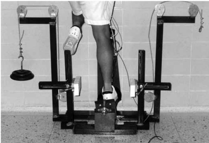
**Figure 1** — Ankle-inversion/eversion strength-training machine with the axis of rotation for ankle inversion/eversion inclined  $42^\circ$  above the dorsum of the foot with an anteromedial deviation of  $23^\circ$  about the subtalar joint. The axis of rotation for the ankle-strength-training machine was aligned at the height of the subtalar joint to allow the subject to freely rotate into inversion and eversion.
