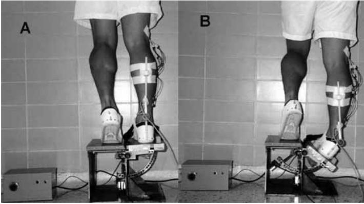
**Figure 6** — Subject standing on the inversion platform (A) before trapdoor release and (B) after the trapdoor was released by an electronic magnetic switch, causing the foot-support base to rotate 37°. An electrical goniometer was rigidly attached to the rear of the shoe and tightly taped to the rear of the subject's lower leg to determine inversion/eversion of the ankle joint.
